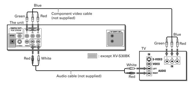
• Connect "Y" to "Y," "PB" to "PB," "PR" to "PR" correctly.
